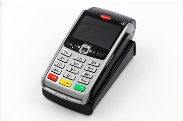
All printing is handled directly by the terminal's on-board thermal printer.
